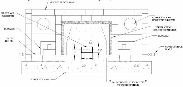
FIGURE 3: OUTSIDE WALL PAD INSTALLATION
